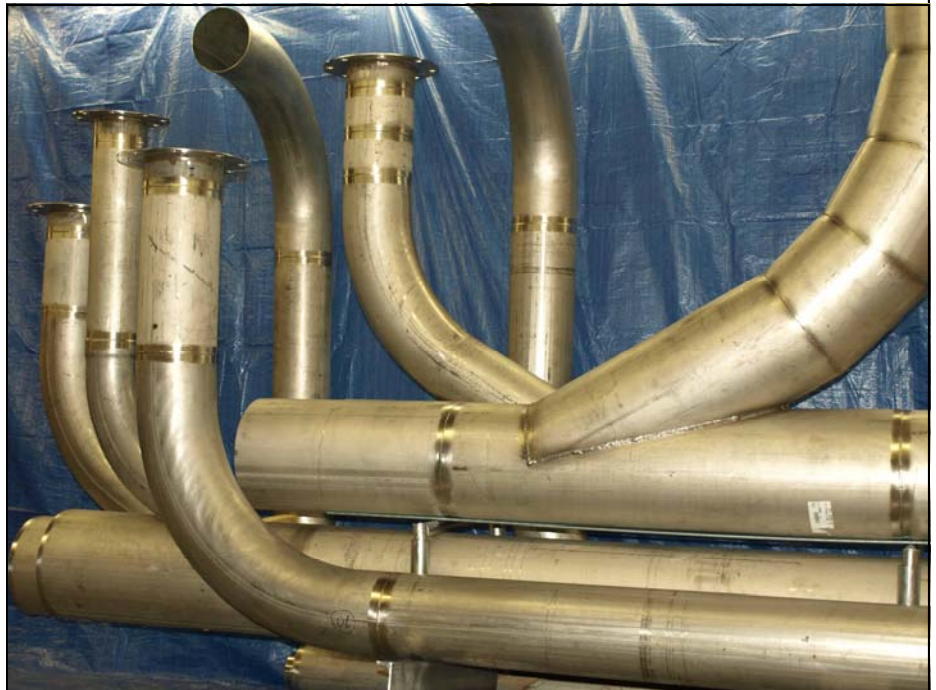
Pre-fabricated, stainless steel process piping is ready for delivery.
