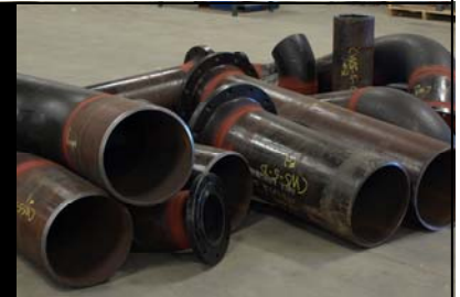
An 8 piece fabricated assembly weighting over 4,000 lbs is easily handled by one man with the use of overhead cranes and rollers.
