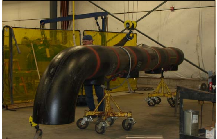
An 8 piece fabricated assembly weighting over 4,000 lbs is easily handled by one man with the use of overhead cranes and rollers.
